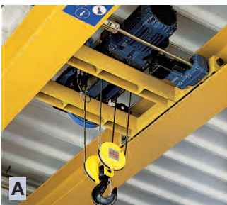
A - Safelift DRH hoist with DRT crab unit on Safelift overhead crane.
