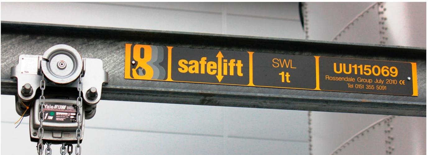
**Selection** Safelift overhead runway beams and rolling beam cranes are available in a range of sizes, capacities and duty classes. Select the runway beam or crane to be used and plan the lift taking into account the capacity, class of use and range of lift. Consult the supplier if the crane is to be used in areas of high risk, exposed to the elements, water, steam etc, with hazardous substances, e.g. acids or chemicals, or subjected to extremes of temperature.
